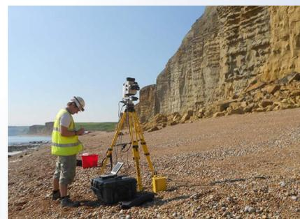
The British Geological Survey's Landslide Response Team map the collapsed cliff from a safe distance using Terrestrial Laser Scanning technology. Taken 25 Feb 2012.
